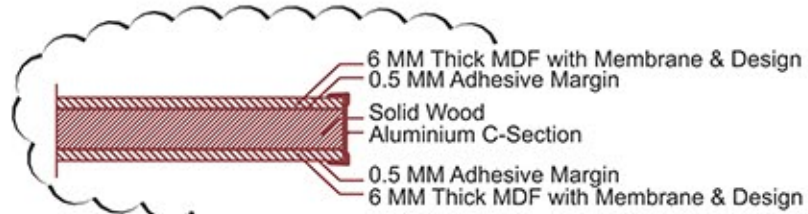
Cut section Detail with Aluminum Beading
